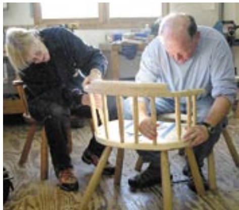
We still use a brace and auger bit to bore the leg-tenon mortises.
