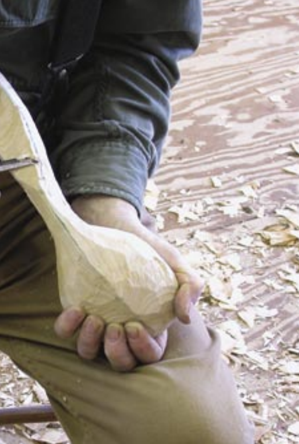
When it comes to carving the end of the handle, work towards the centre, from the edge, with a slicing action achieved by rotating your wrist. The thumb acts as a pivot
