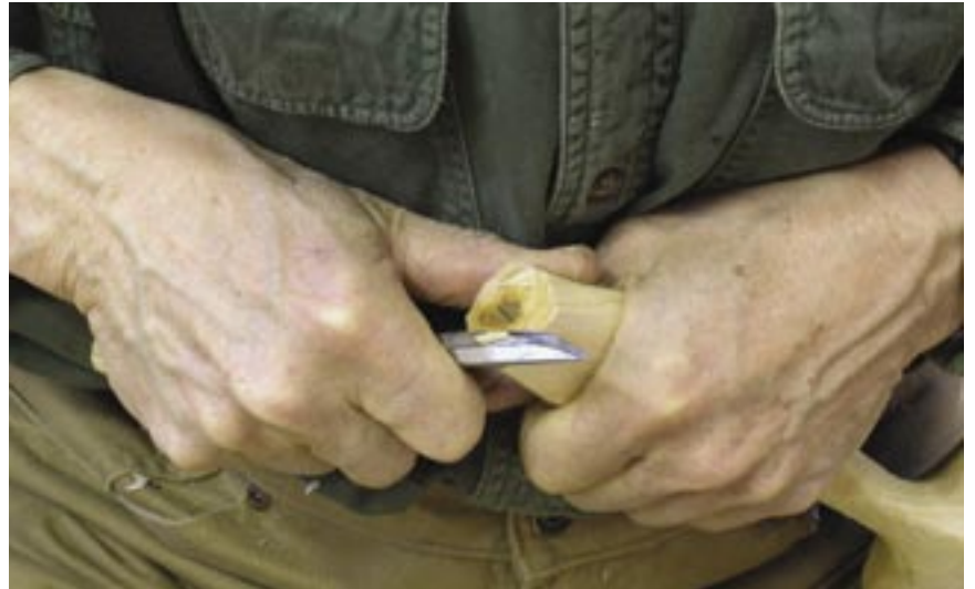
When it comes to carving the end of the handle, work towards the centre, from the edge, with a slicing action achieved by rotating your wrist. The thumb acts as a pivot
