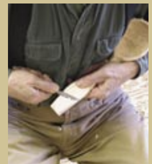
When carving the tablets, Drew cuts with a scissors action, working away from his body, clutching the ladle in the crook of his elbow. How you hold the workpiece is as important as the holding of the knives.
